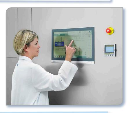
As option, the unit is supplied with our complete SCADA control system PharmaSter®. This system includes an industrial PC with touch-screen colour display. The software allows not only for supervision and control of the process, but also compiling, storing and processing the whole information in a batch oriented mode. The system is fulfilling 21 CFR Part 11 guidelines.
