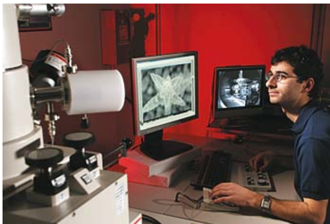
Scanning electron microscopes, like the one shown here, can “see” details as small as one nanometre – one millionth of a metre!
