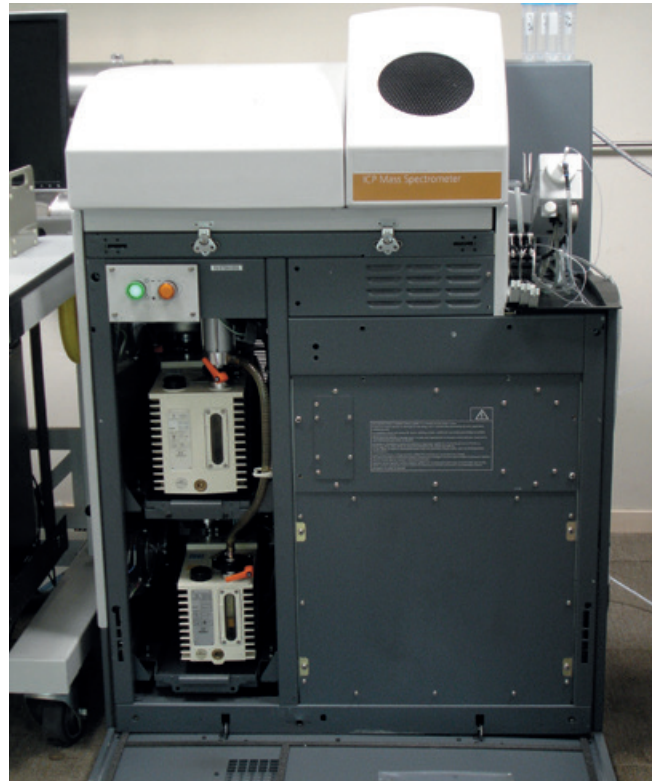
ICP-MS. Photo courtesy Agilent Scientific Instruments.
