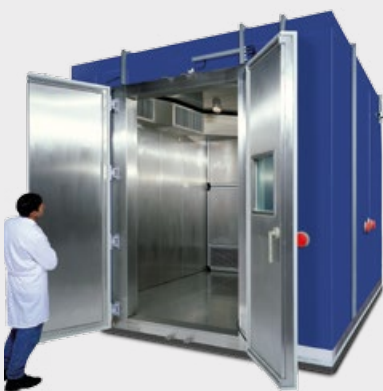
Walk-in chamber equipped with indirect cooling system to test specimen (base station) with high heat dissipation
