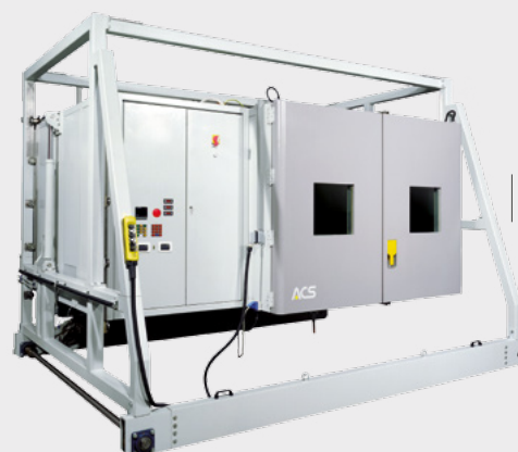
Vibration chamber (capacity 6000 lt approx.) to simulate combined stress (temperature, humidity, vertical and horizontal vibration) on vehicle devices
