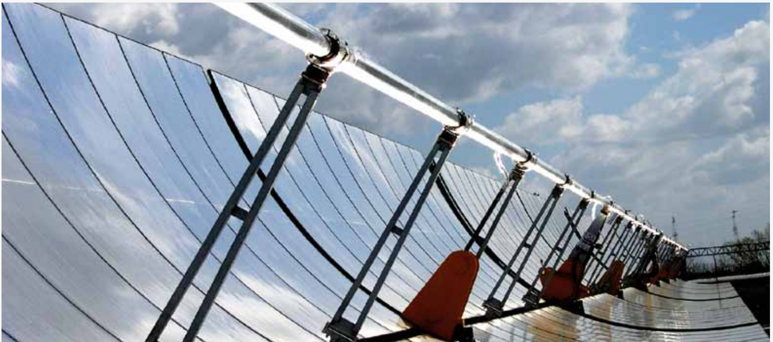
“Parabolic troughs (CSP technology-Concentrated Solar Power) with solar receiver tubes manufactured by ASE, Archimede Solar Energy of Angelantoni Group”
